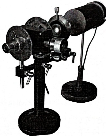
Figure-7: Babinet compensator experimental set-up using white light
